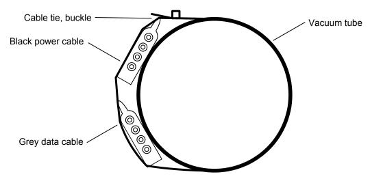
Note: When approaching a node location, stop the attachment process. Run the cables over the node area (such as a T-valve) and make sure you create a slight amount of slack when continuing the attachment with cable ties. Doing so lets you install KwikLink connectors or ArmorBlocks with greater ease, with less stress on the cable.
